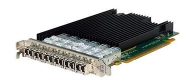
The Silicom 10GB NIC Ethernet PCI Express Network Interface Cards are based on Intel 82599ES Ethernet controller with two fully integrated Gigabit Ethernet Media Access Control (MAC) and SFI ports.
