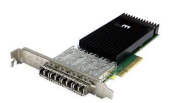
The Silicom 10 Gigabit Ethernet PCI Express server adapters are based on Intel XL710 Ethernet controller with fully integrated Gigabit Ethernet Media Access Control (MAC) and SFI Interface. In addition to managing MAC and PHY Ethernet layer functions, the controller manages PCI Express packet traffic across its transaction, link, and physical/logical layers. Using hardware acceleration, the controller offloads tasks from the host, such as TCP/UDP/IP checksum calculations and TCP segmentation.
