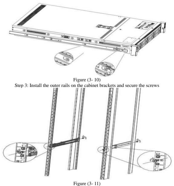
Note: When installing the guide rail, it is necessary to align with the U mark, and when it is installed in place with a snap, secure it with M5 screws.
