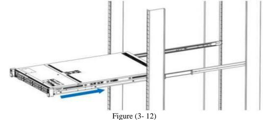
Note: When you push the chassis forward, you will hear a snapping sound. If you can't push it, you need to pull down the buckle of the inner rail to continue to push the chassis gently.
