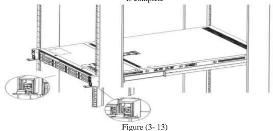
Note: During equipment maintenance, it is necessary to loosen the panel screws and pull the chassis lightly. Do not push or pull the chassis at random speed to avoid damage to the equipment.
