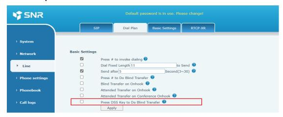
After adding a number to the memory key and pressing the transfer key, you can press this key to transfer the call to the third party.
