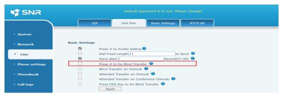
Select **Press** # to **Do Blind Transfer**, enter the number on the transfer dialing interface, and press # to perform blind transfer. If you do not select this option, the phone does not perform blind transfer after you press #.
