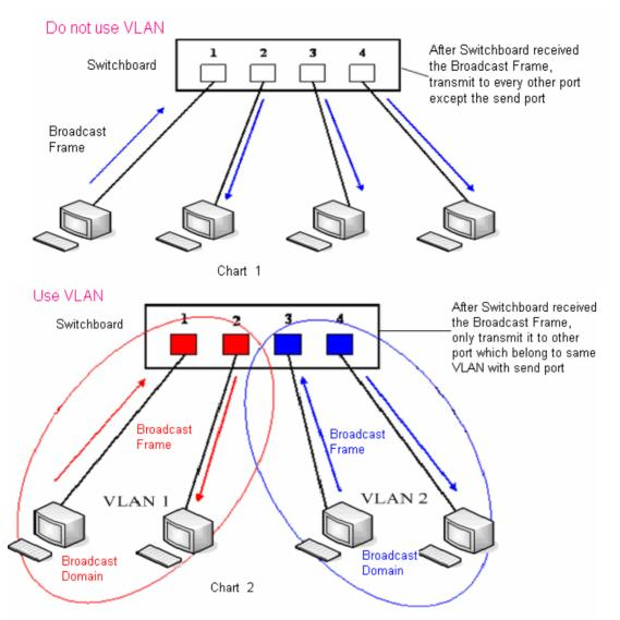
In chart 1, there is a layer 2 switch without setting VLAN. Any broadcast frame will be transmitted to the other ports except the send port. For example, broadcast information is sent out from port 1 then transmitted to port 2, 3 and 4.
