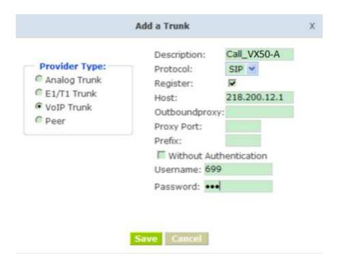
The general environment for two ZPX50 IP PBX in different location and one or both two are behind router and using the private IP. So we need to make port forwarding in the router and make SNR-VX50 IP PBX reach to each other.
