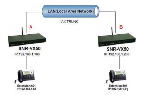
Register the SNR-VX50-A as an peer in SNR-VX50-B(via SIP trunk), so the extensions in SNR-VX50-A can make calls to SNR-VX50-B's extensions via this "special" trunk. In above structure:
