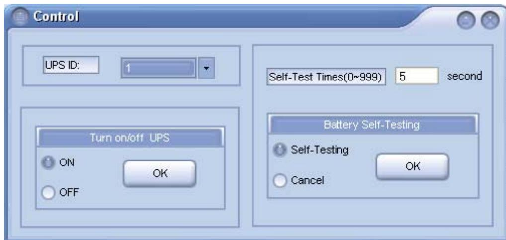
Users can select Turn on/off UPS, Battery self-testing, Cancel self-testing.
