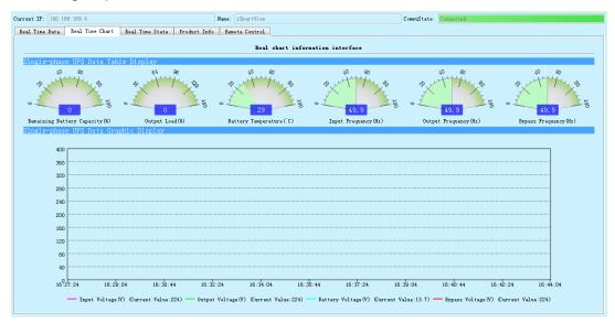
Single phase display interface including residual capacity of the battery, load
