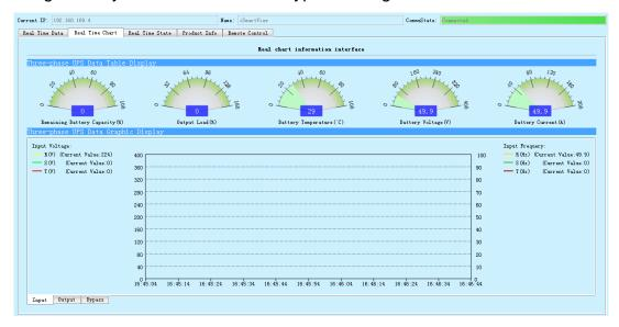
Three phase display interface including residual capacity of the battery, load percentage, battery temperature, input and output frequency and chart information of bypass frequency, as well as input and output voltage, battery voltage and dynamic curve chart of bypass voltage.
