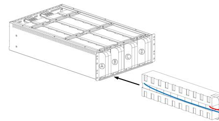
**step 5:** assemble the inner panel, all cables cross through the holes on panel as below
