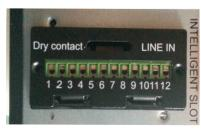
4. Connect with monitoring device by connecting wire of dry contact card. The monitoring device will display and control UPS operating status, to achieve remote monitoring of UPS operation.
