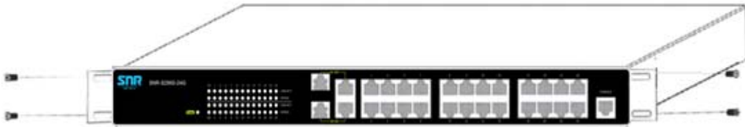
Fig 2-1 Fasten the Brackets to the Switch
