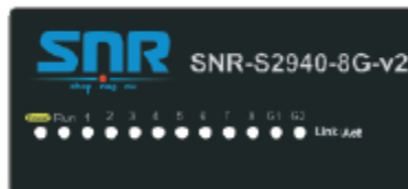
Fig 1-4 SNR-S2940-8G-v2 LED diagram
