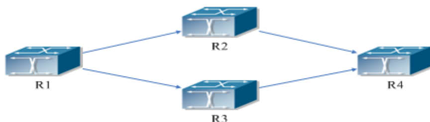
Figure 4-17 the application environment of ECMP
