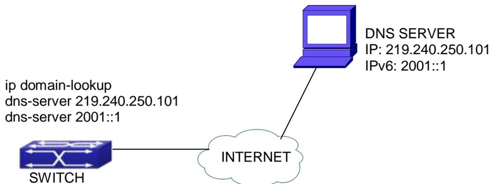
Fig 3-1 DNS CLIENT typical environment
