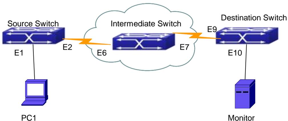
Fig 2-1 RSPAN Application Sample
