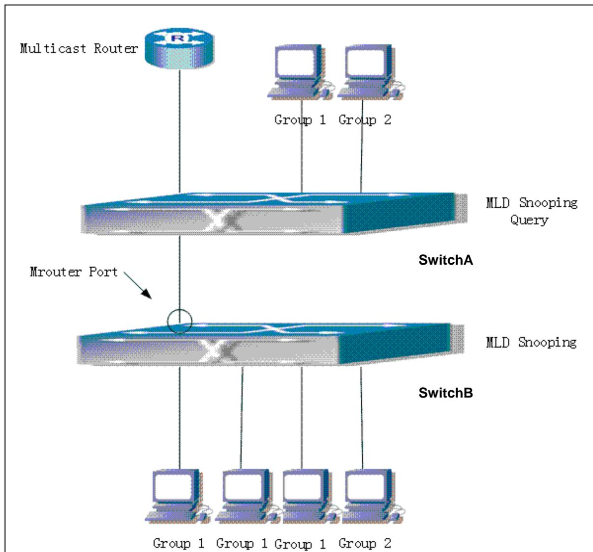
Fig 2-7 Switch as MLD Querier Function figure
