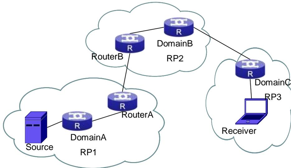
Fig 1-3 Network Topology for MSDP Entry
