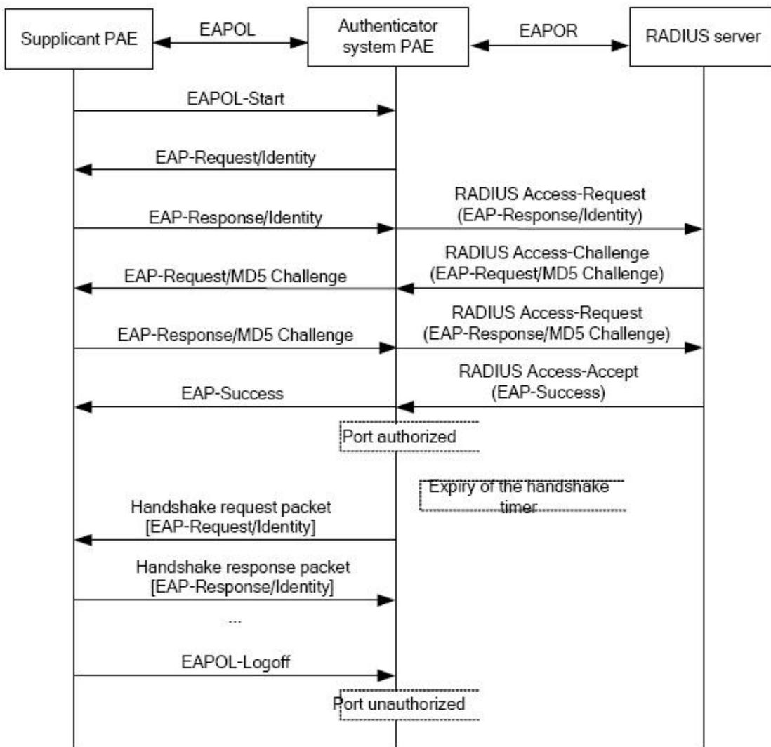
Fig 2- 10 the Authentication Flow of 802.1x EAP-TLS
