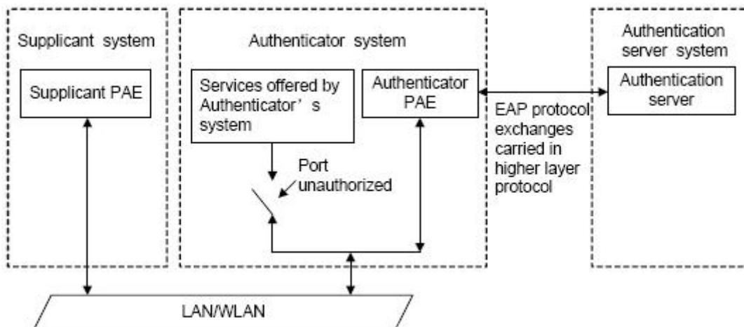
Fig 2- 1 The Authentication Structure of 802.1x
