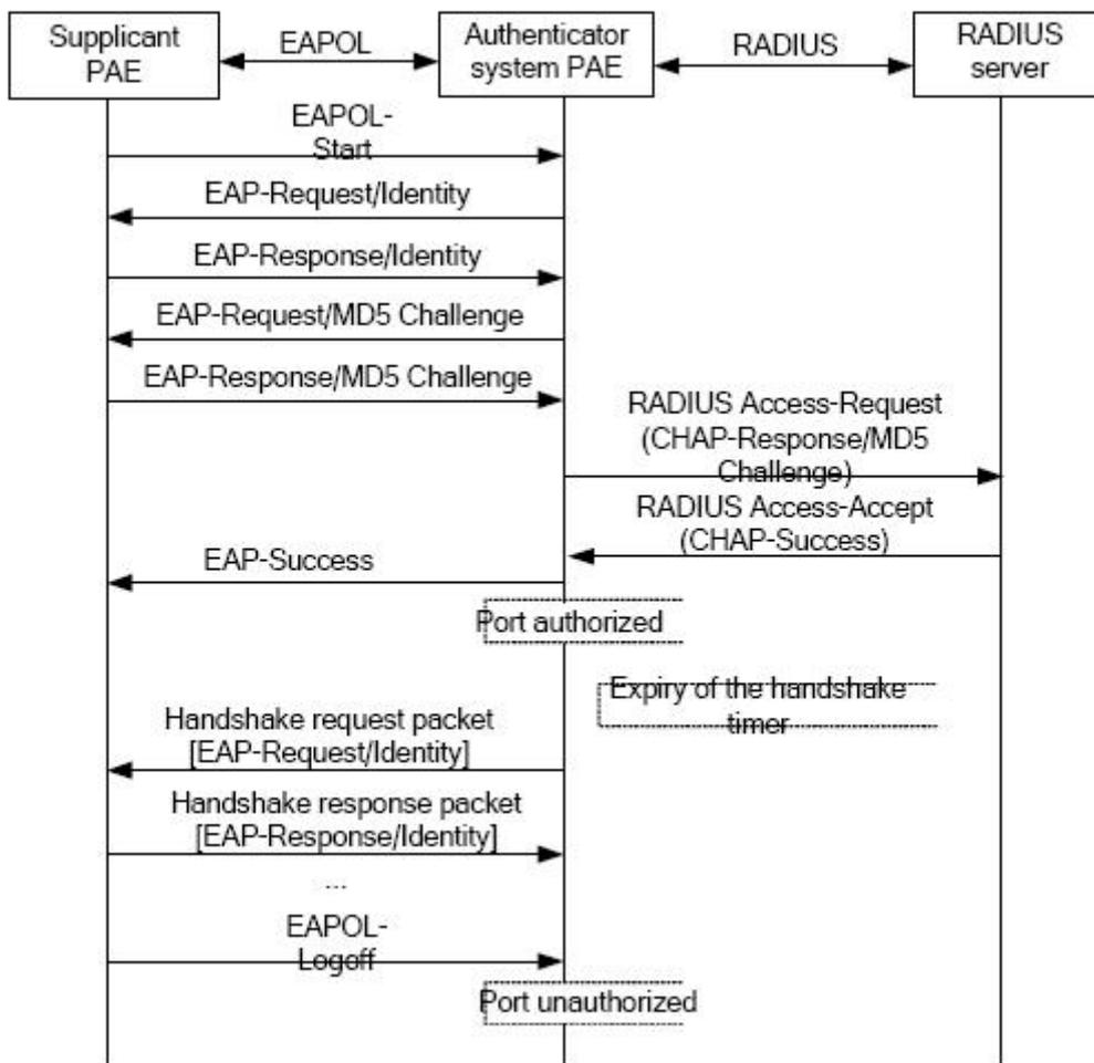
Fig 2- 12 the Authentication Flow of 802.1x EAP Termination Mode
