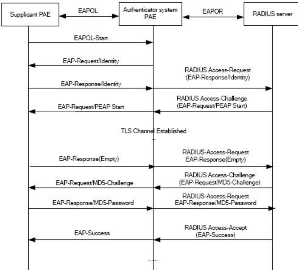
Fig 2- 11 the Authentication Flow of 802.1x PEAP
