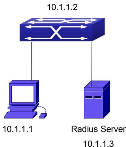
Fig 2- 16 IEEE 802.1x Configuration Example Topology
