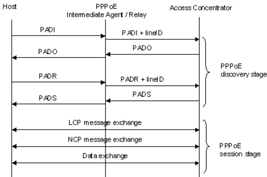
Fig 11- 1 PPPoE IA protocol exchange process
