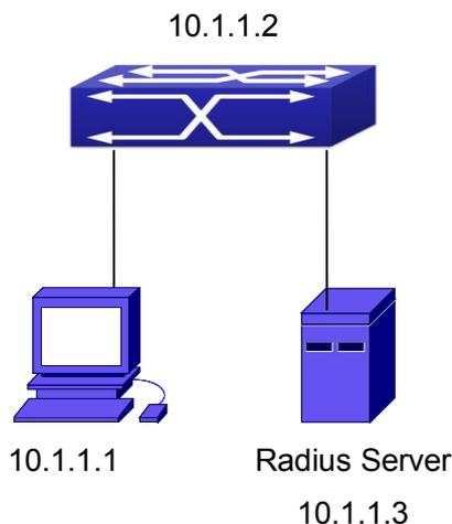
Fig 6- 2 The Topology of IEEE802.1x configuration
