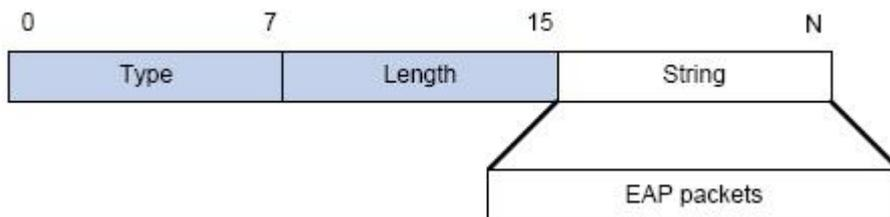
Fig 2- 6 the Encapsulation of EAP-Message Attribute
