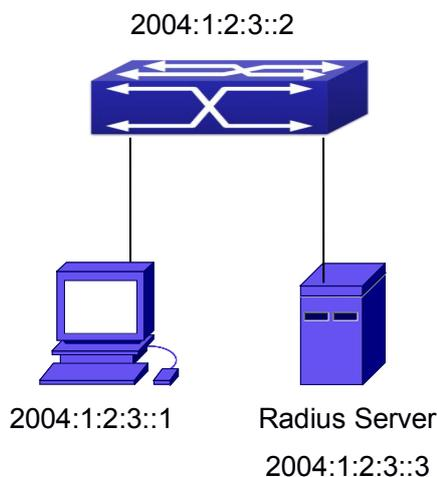
Fig 6- 3 The Topology of IPv6 Radius configuration
