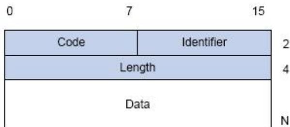
Fig 2- 4 the Format of EAP Data Packets
