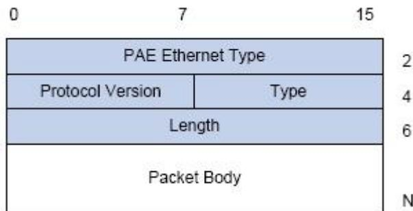
Fig 2- 3 the Format of EAPOL Data Packet
