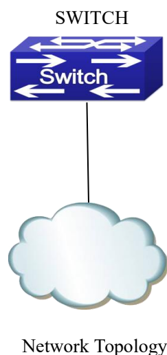
Figure 2-3 Typical example of port loopback detection
