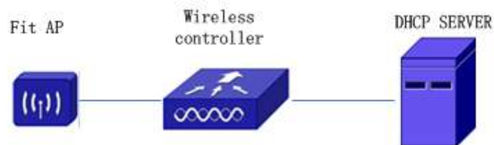
Fig 4-1 Typical DHCP option 60 and option 43 topology
