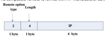
IP means the primary IP address of layer 3 interface where DHCP packets from.
