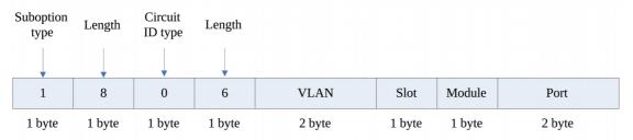
The VLAN field is written with the switch VLAN ID. For the rackmount switch, Slot means the slot number; for the cassette switch, it is 1. The default module is 0. Port means the port number and starts from 1.
