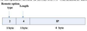
IP means the primary IP address of layer 3 interface where DHCP packets from.
