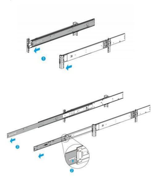
Step 3. Install the inner rails to the chassis (the left and right inner rails are the same, please repeat the installation)
