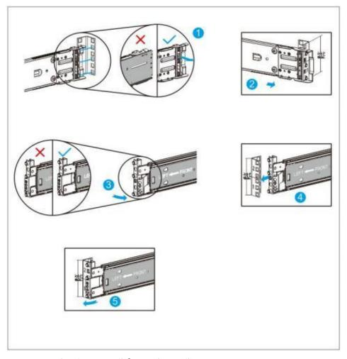
Step 2. Remove the inner rail from the rail
