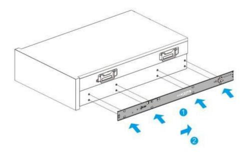
Step 4. Install the server into the rack.
