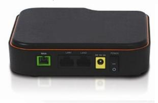
SNR-ONT-2G is G-PON Optical Network Terminal (ONT) compliant with ITU-T G.984 standards. SNR has developed SNR-ONT-2G for all clients on the basis of G-PON technology. G-PON technology supports upstream 1.25Gbps and downstream 2.5Gbps PON transmission rate, highly efficient bandwidth usage for Ethernet multi-services and ensures that the carrier can provide reliable quality of services to their customers.
