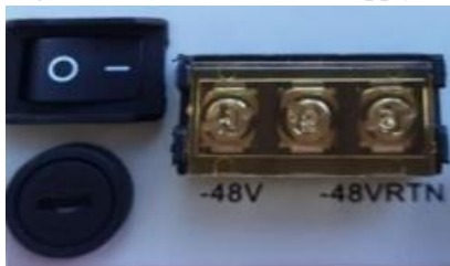
Figure 3-4 -48VDC Power Supply PIN Definition
