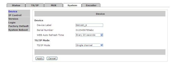
**Device Label:** Check the name and the serial number of this device. User can resign this product name at will, the device name should be less than 24 characters. The serial number is read-only.
