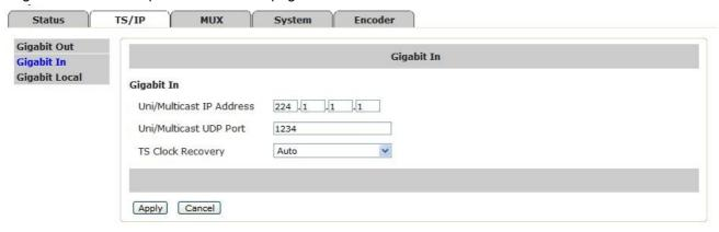
**Uni/Multicast IP Address:** set the multicast address for the incoming IP streaming. To receive a unicast streaming, the submenu can be ignored.
