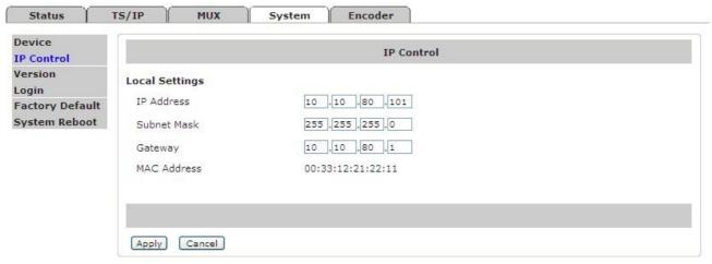
IP Address: set the device's IP address
