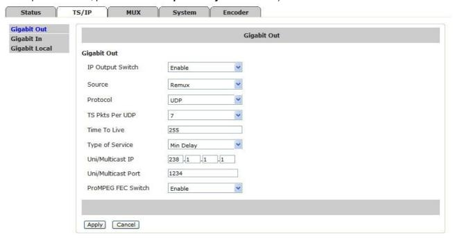
IP Out Switch: Enable or Disable the IP output
