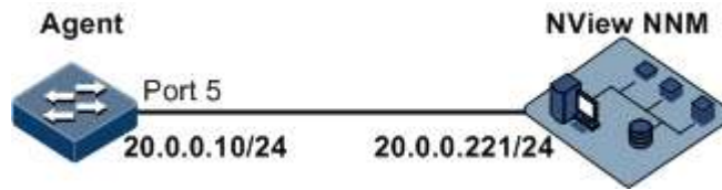
Figure 10-3 SNMP v1/v2c networking
