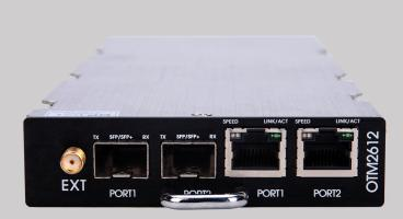
OTM2612 10G Packet Ethernet/SDH/OTN Test Module is a multi service test solution for the installation and maintenance for Metro/Carrier Ethernet, IP services, SDH/SONET, OTN circuit test up to 10G. Not only does it supply a compact test solution for 10G packet Ethernet, include ITU-T Y.1564 Standard for SLA test features, but also for SDH/SONET supports Out-of Service test, Round Trip Delay, In-service test, overhead controlling and decoding, troubleshooting, APS timing etc.
