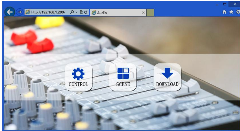
Control: Control channel parameters and the opening and closing of each processor.
