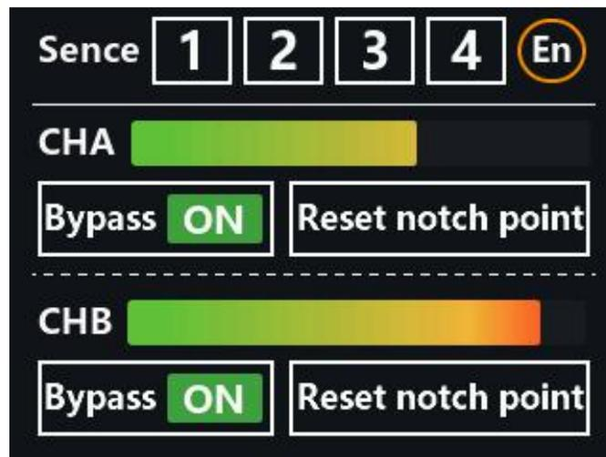
This interface mainly includes scene switching, signal level display, channel bypass, reset notch point, screen lock, language switching.
