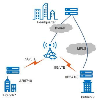
Huawei NetEngine AR6710-L series routers feature 5G/LTE functionality, enabling wireless interconnection between enterprise branches and between the headquarters and branches. A 5G/LTE link can function as the active link or as a backup for wired links, enhancing network stability while reducing network construction cost.
