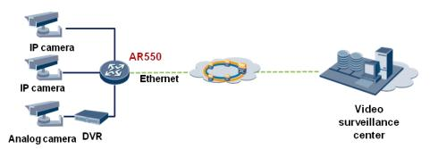
Video surveillance is popular in various industries. Different access conditions pose higher requirements on the installation space and mode, operating temperature and humidity of video backhaul devices. The AR550 uses a compact design and has a
