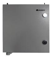
F01A109 is outdoor low-voltage distribution cabinet for AR550. Power distribution cabinet is equipped with one 60W open frame power supply, one-circuit 220VAC/10A/2P miniature circuit breaker for input, one power lightning arrester and two four-port anti-lightning boards, which provide safe and reliable protection for the entire distribution and communication system.
