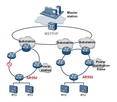
The AR550 supports the SEP protocol to ensure highly reliable network communication by implementing fast protection switching. It complies with IEEE1613 and IEC61850-3 substation environment standards and can be used in power distribution automation and automatic substation access scenarios, boosting digital and smart development of the electric power industry.
