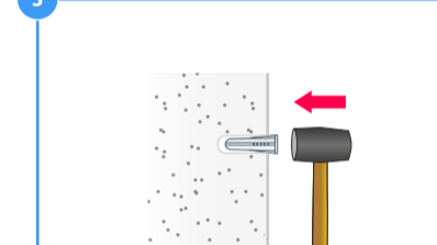
Hammer a screw anchor into each hole.
