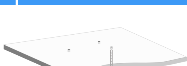
Remove the ceiling tile and mark installation holes. Drill three holes in the ceiling tile.
