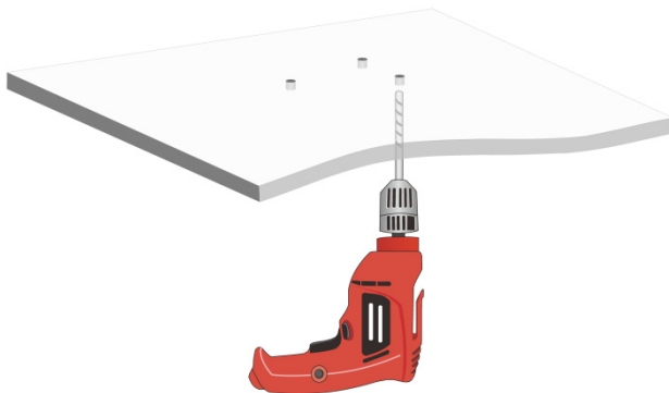
Figure2-7 Drilling holes in the ceiling tile
