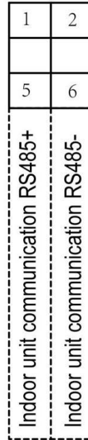
Figure 2-23 Schematic diagram of indoor unit communication wiring
