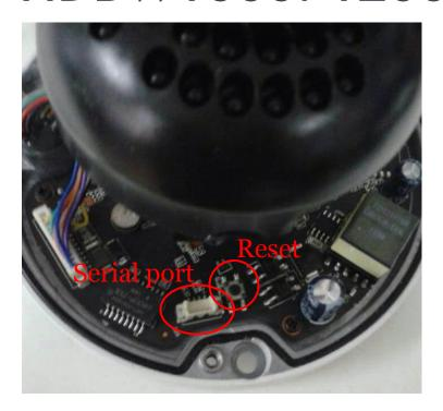
Reset: Press the reset button for 5 seconds.
