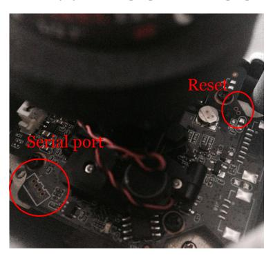
Reset: Make short circuit between two small holes on the PCB for 5 seconds.
