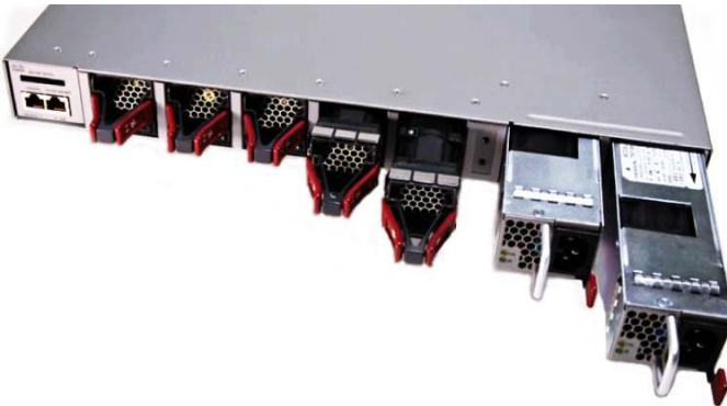
Figure 7. Redundant Fan and Power Supply
