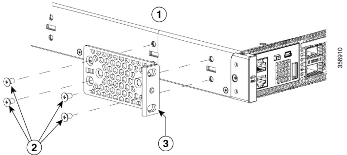
**Figure 31: Middle Mounting position of Rack Mounting Brackets**
