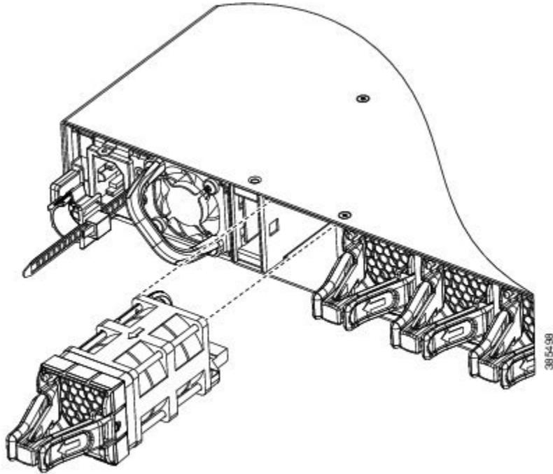
*Figure 64: Installing the Fan Module on Cisco Catalyst 9500 High Performance C9500-32C Switch Model*
