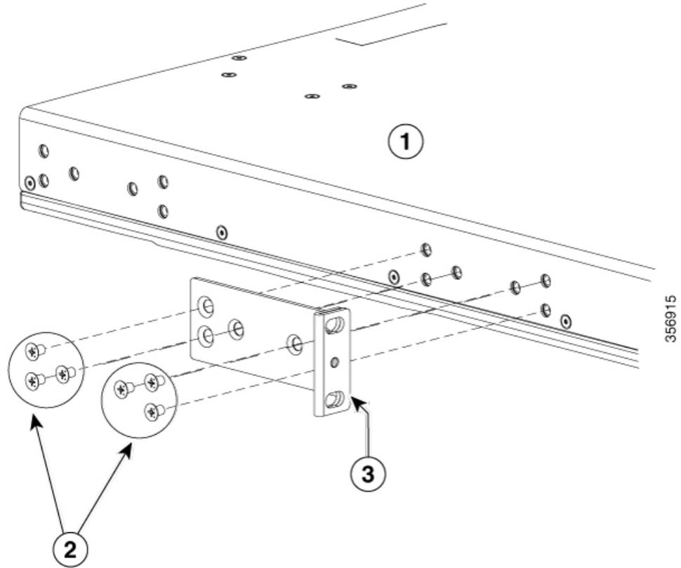
Figure 35: Rear Mounting position of Rack Mounting Brackets
