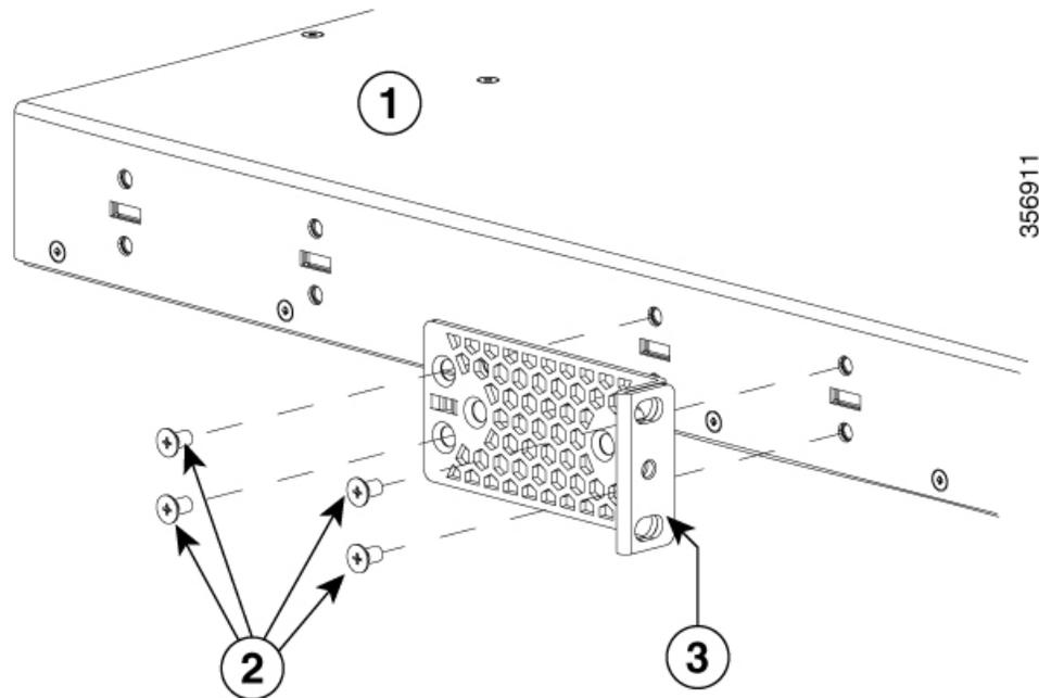
Figure 32: Rear Mounting position of Rack Mounting Brackets
