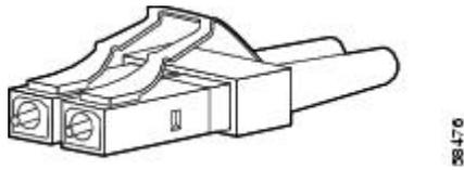
Figure 81: Simplex LC Cable Connector
