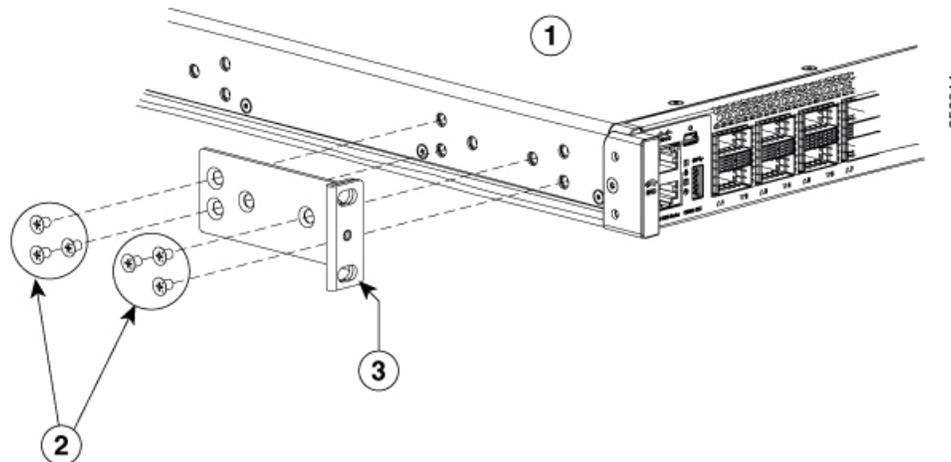
Figure 34: Middle Mounting position of Rack Mounting Brackets
