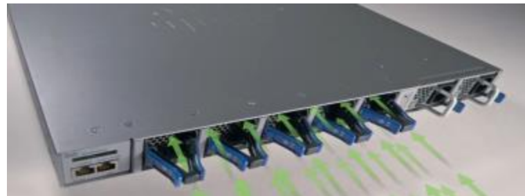
Blue color fan and P/S handles for back to front airflow
