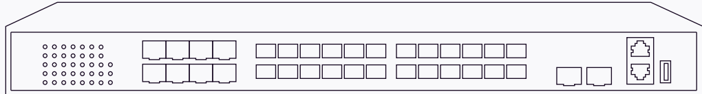
S300X-24FQ Stackable 10GE L3 switch with 1GE RJ-45, 1/10GE SFP+, and 40GE QSFP+ ports. Supports dynamic routing protocols: OSPF, BGP, RIP, PIM, MSDP. Capable of handing up to 16K IPv4 and 8K IPv6 routes, 16K ARP entries, 4K multicast groups, and 32K MAC addresses.
