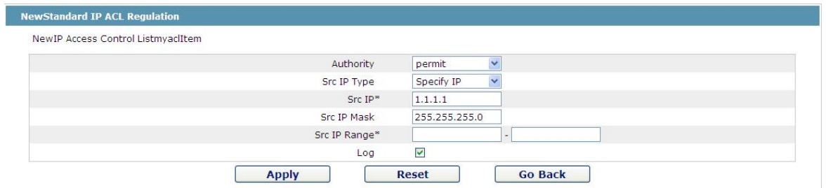
Figure 12: Setting the Rules of the standard IP access control list
