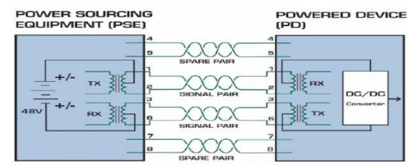
Generally speaking, standard PD has to support two power reception modes, while PSE only needs to support one of the two modes. All MY COMPANY products, as the PSE switches, only support the signal line power supply—alternative A.
