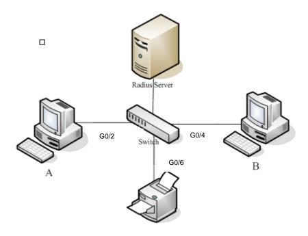
Host A connects port G0/2 of the switch. Host B connects port G0/4. Host C connects with port G0/6. The IP address of the radius-server host is 192.168.20.2. The key of radius is TST. Port G0/2 adopts remote radius authentication, user binding and re-authentication. Port G0/4 adopts local authentication of eap type, and enables multi-host and guest-vlan. Port G0/6 adopts mab authentication and the mac address format is AA:BB:CC:DD:EE:FF.
