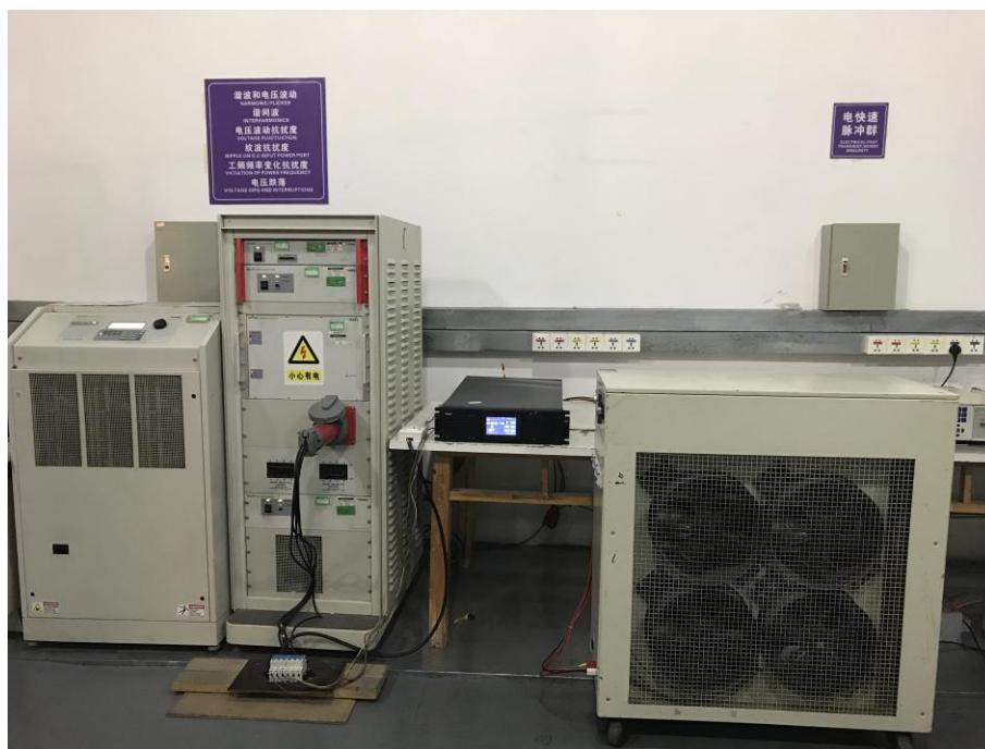
18.11.Photo of Low Frequency Signals and Power Line Unbalance Test
