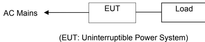
5.1.2. Block diagram of test setup (In chamber)
