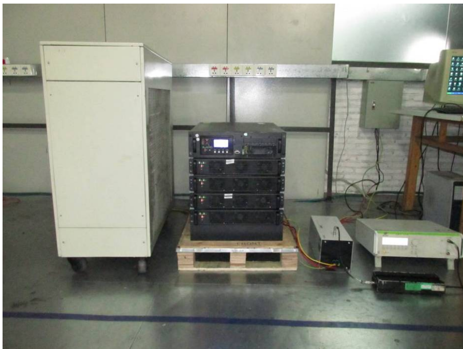
16.9.Photo of Injected Currents Susceptibility Test
