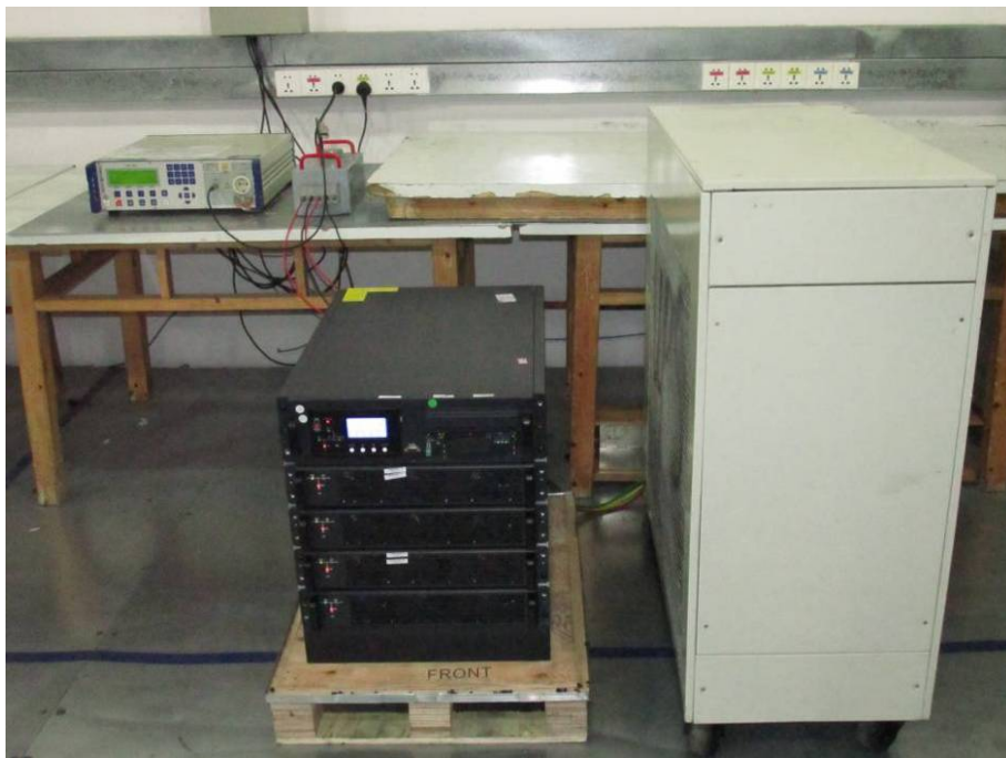
16.7.Photo of Electrical Fast Transient / Burst Test
