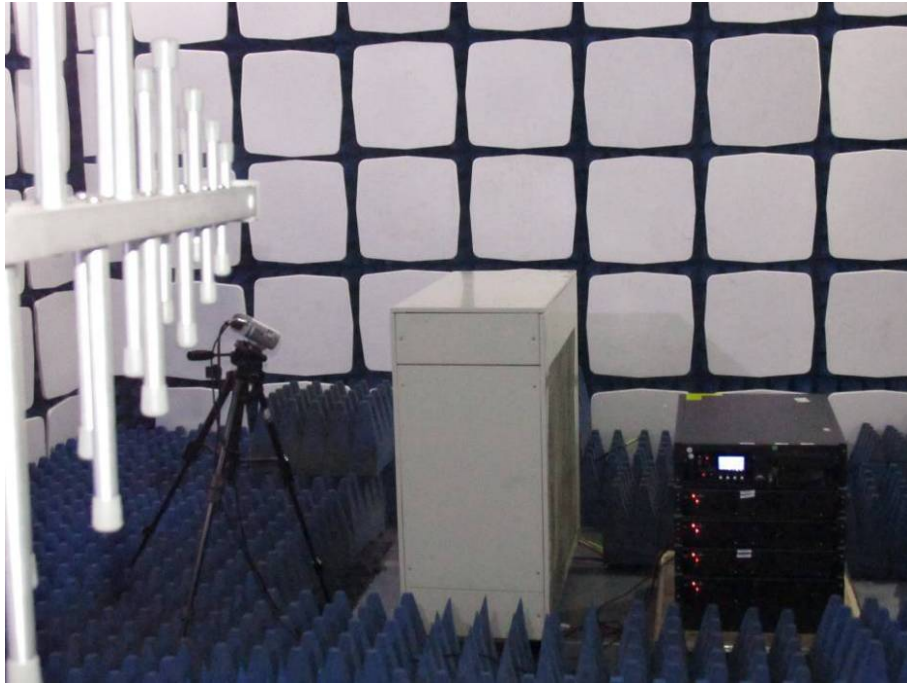
16.6.Photo of RF Field Strength Susceptibility Test
