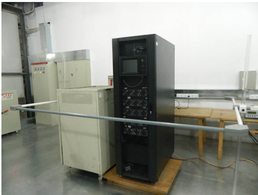
16.9.Photo of Magnetic Field Immunity Test
