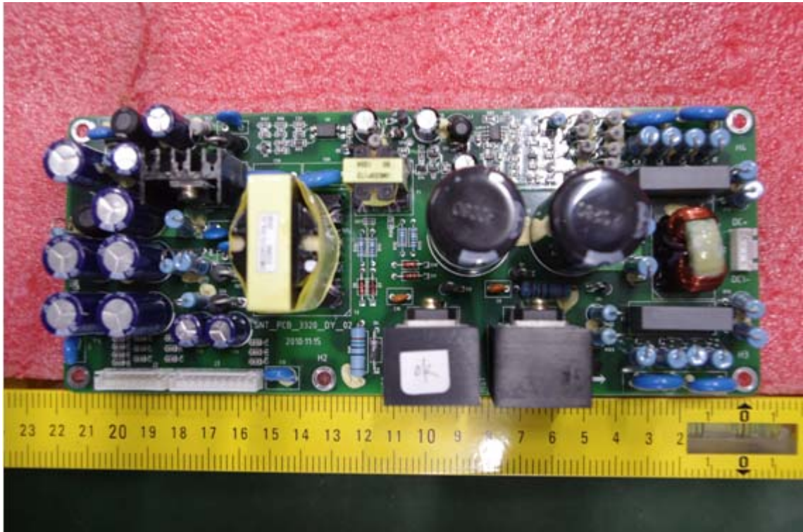
Fig. 7 – Board SNT_3320_PCB_DY, components side view
