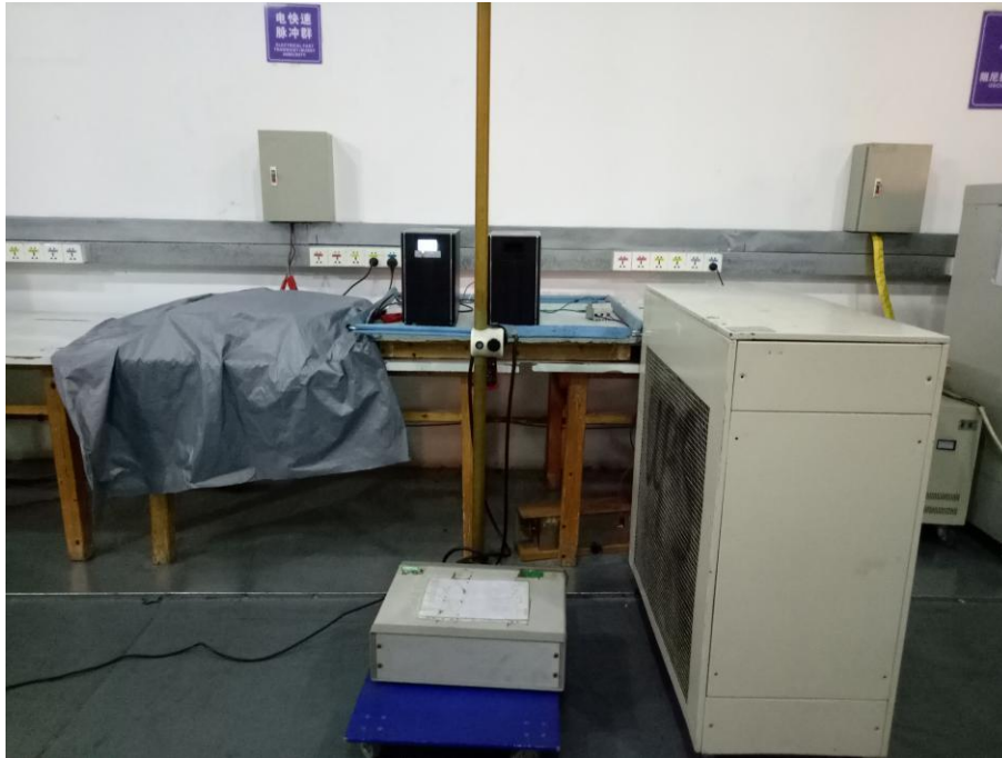
17.9.Photo of Magnetic Field Immunity Test
