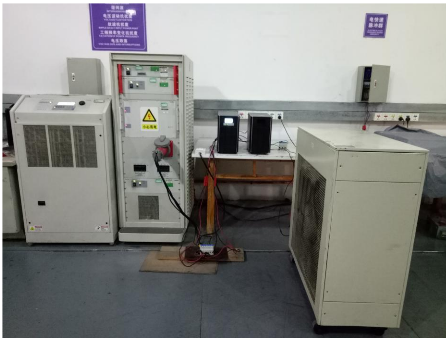
17.10.Photo of Voltage dips and interruption Test
