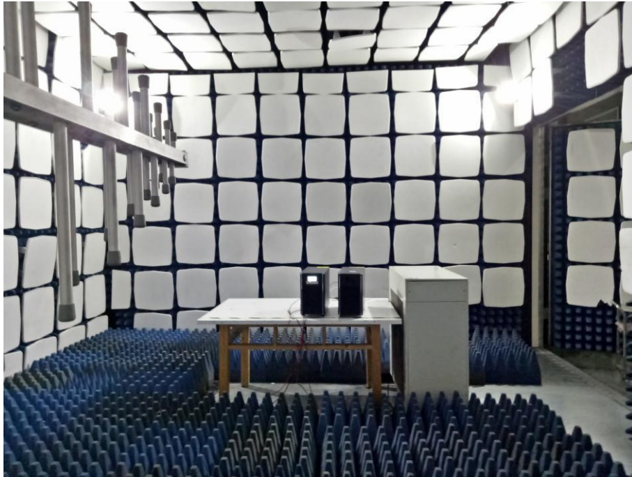
17.5.Photo of RF Field Strength susceptibility Test
