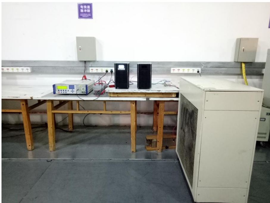
17.6.Photo of Electrical Fast Transient/Burst Test
