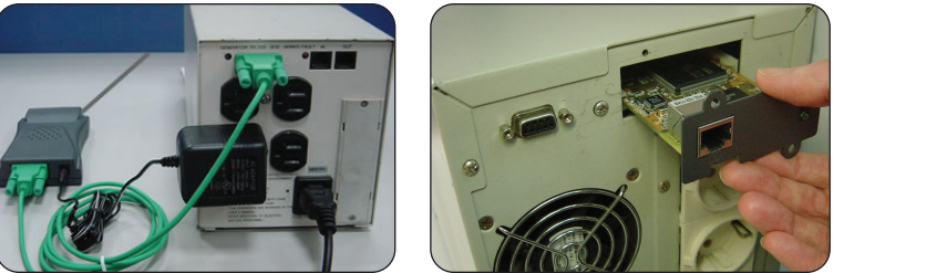
NetAgent II - External Card Installation NetAgent II - Internal Card Installation
